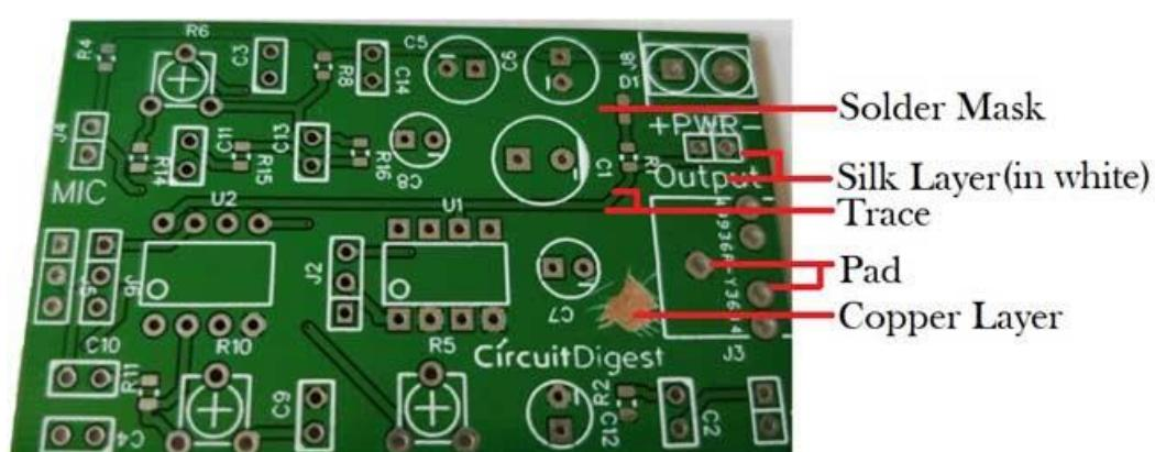
**Pad:** Pad is nothing but a piece of copper on which lead of components are mounted and on which soldering are done. Pad provides the mechanical support to the components.
