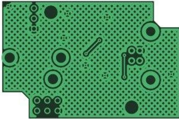
One of the downsides of a plane is the difficulty to solder a component, since the heat gets dissipated quickly through the plane. To avoid this, the contacts to planes can be made through thin traces, like the picture below.
