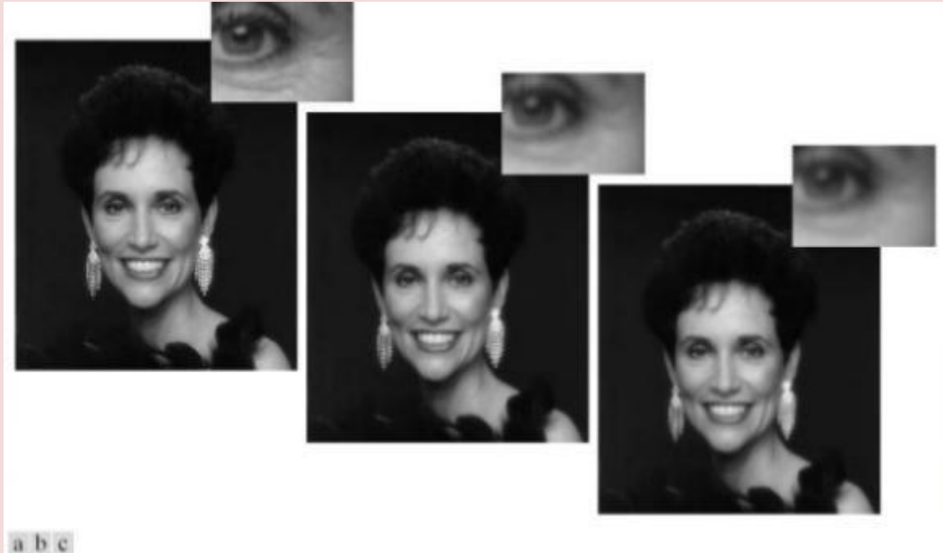
Fig. (a) Original image (784x 732 pixels). (b) Result of filtering using a GLPF with D0 = 100 . (c) Result of filtering using a GLPF with D0 = 80 . Note the reduction in fine skin lines in the magnified sections in (b) and (c).
