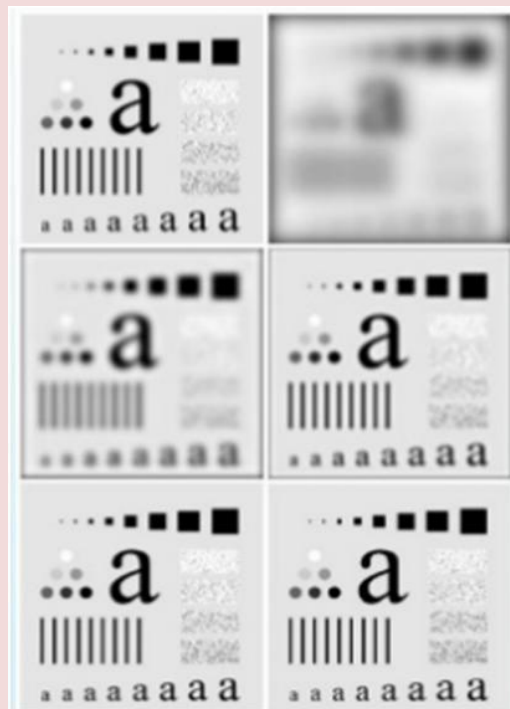
Fig. (a) Original image. (b)-(f) Results of filtering using BLPFs of order 2, with cutoff frequencies at the radii
