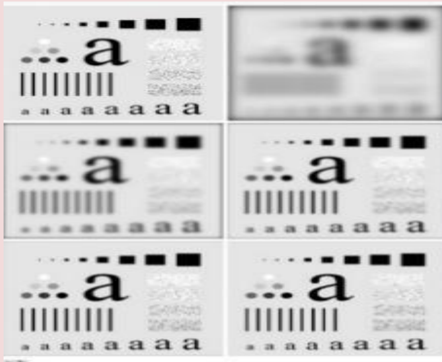
Fig.(a) Original image. (b)-(f) Results of filtering using GLPFs with cutoff frequencies at the radii shown in fig.2.2.2. compare with fig.2.2.3 and fig.2.2.6
